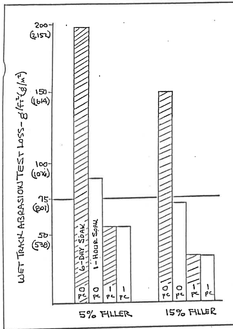
FIG. 16. EFFECT OF FILLER & CEMENT CONTENT ON 1-HOUR & 6-DAY SOAK WET TRACK ABRASION TEST LOSS - 12% EMULSION
