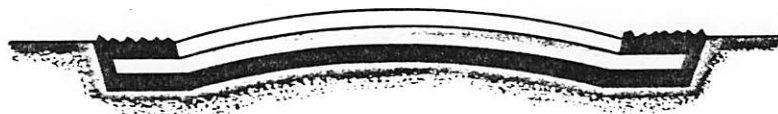
McAdam's simple but effective road pavement consisted of wearing surface and base course comprising three layers of 5-cm. stones laid on a compacted cambered footing.
